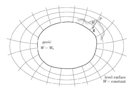
Figure 1. Level surfaces and plumb lines (Hofmann-Wellenhof and Moritz, 2005).
